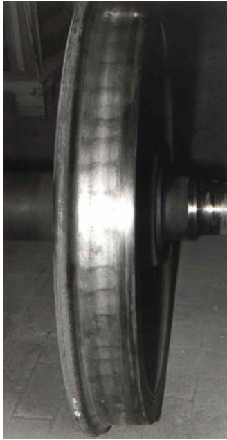
Fig. 1. The wear area of the contact effect analysed by the authors
