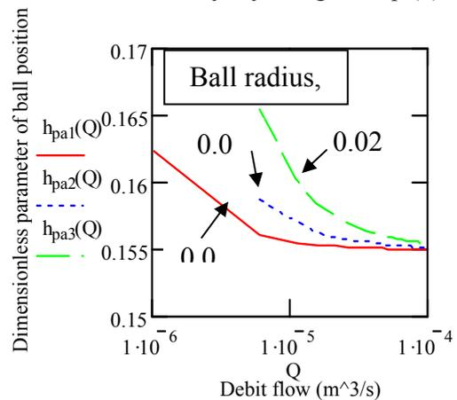
Fig. 2. Position ball in conical gape
