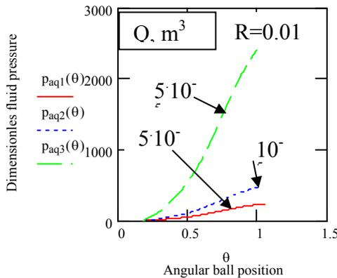
Fig.4. Fluid pressure in gap for diverse flow rates
