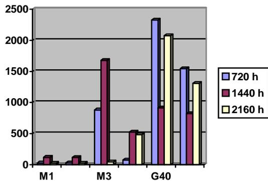
Fig. 12. Corrosion rate of ball and seat materials
