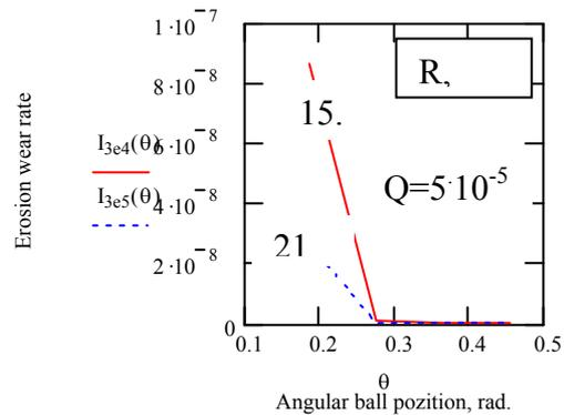
Fig.8. Erosion wear rate vs. angular ball position and ball radius
