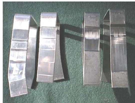
Figure 3: The appearance of the test piece after multiple drawing
