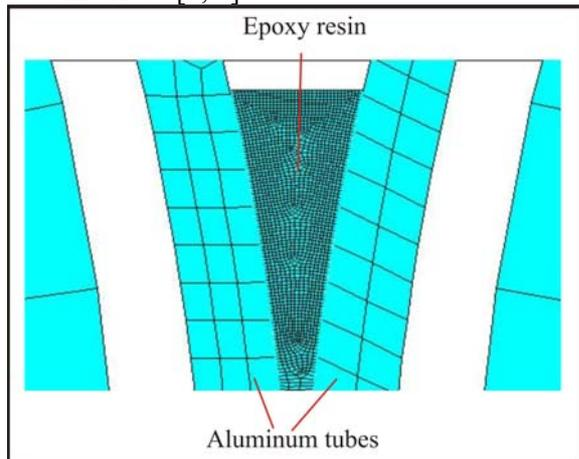
**Figure 10:** Detail of the FEM model in the region of the resin and aluminium contact
