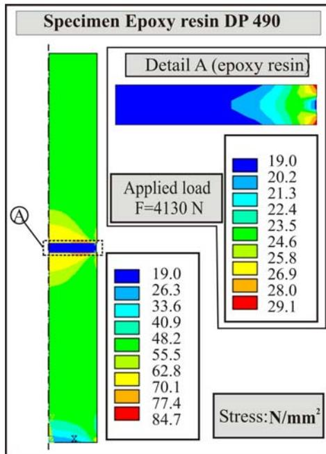
**Figure 4:** Typical FEM simulation results of the tensile loading for the cylinders bonded with various epoxy resins.
