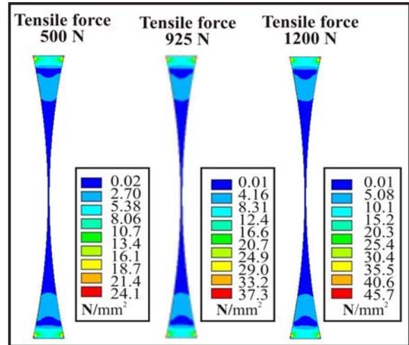
**Figure 11:** von Mises equivalent stress distribution under 500, 915 and 1200 N.
