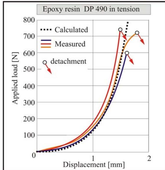
**Figure 8:** Theoretical and measured results of the epoxy resins DP 490.
