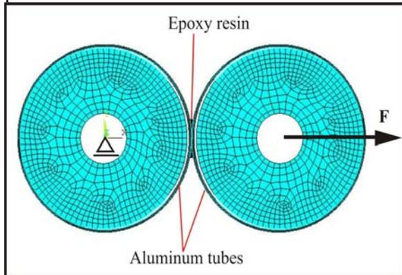
**Figure 9:** FEM model of the glued tubes assembly
