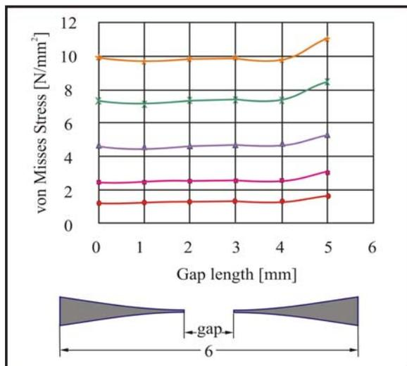
**Figure 13:** The maximum developed von Mises equivalent stress for removed resin region 0 up to 5 mm at various loads
