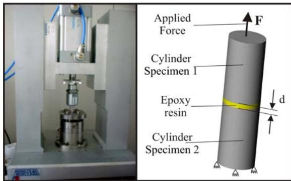
**Figure 1:** Experimental set-up for the tensile loading of glued specimens by epoxy resins.
