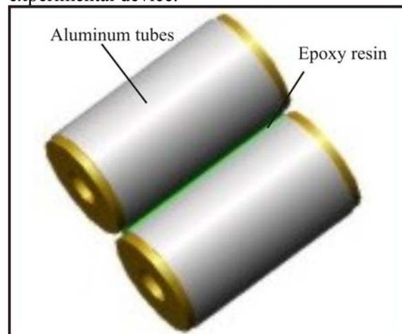
**Figure 5:** Glued specimens of the tensile strength test.
