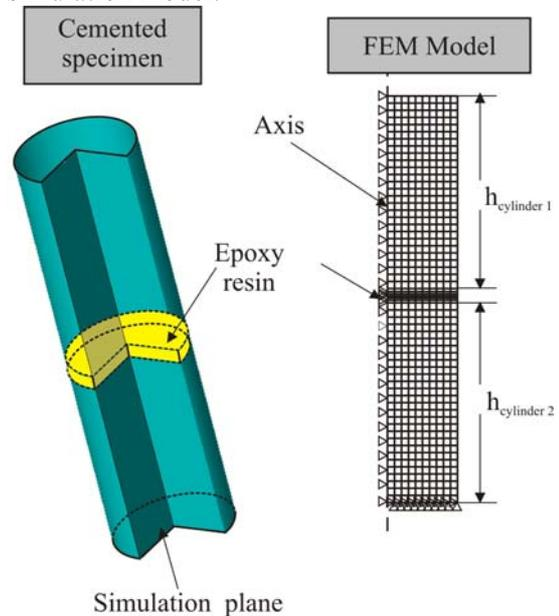
**Figure 3:** FEM simulation model of the glued cylinders' tensile test.
