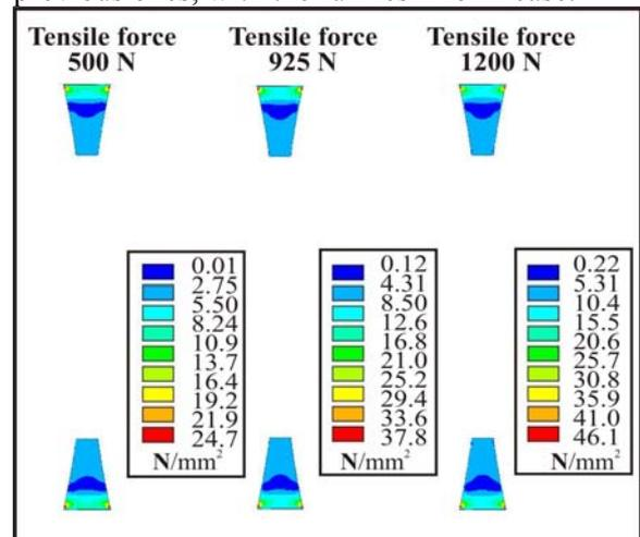
**Figure 12:** von Mises equivalent stress distribution under 500, 915 and 1200 N, and removed resin region of 4 mm.
