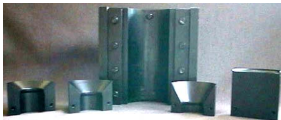
Figure 2 - Die and inserts for axisymmetrical modelling of forward extrusion process
