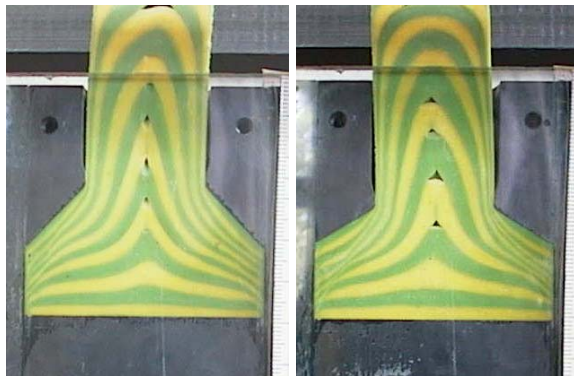
Figure 5 - Plasticine models with central burst defects, lubrication with thicker layer of talc on the specimen and die
