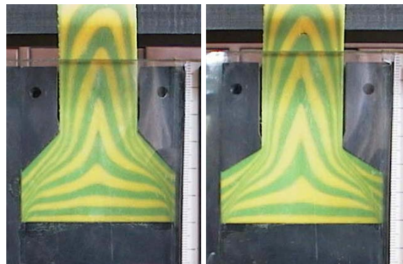
Figure 8 - Plasticine models without central burst defects, lubrication with thinner layer of talc on die surfaces only
