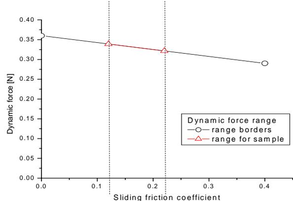
**Fig. 4:** Contact force dependence on sliding friction coefficient
