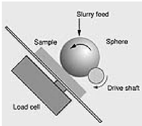
**Fig. 2:** Calowear device principle [4]
