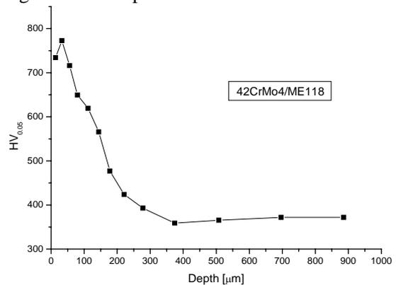
**Fig.1: Hardness depth profile of nitrided sample**
