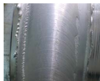
Fig.6: The outer welding surface of tubes according to the varying speeds of stirrer at a constant rotational speed, 2.87 mm/s.
