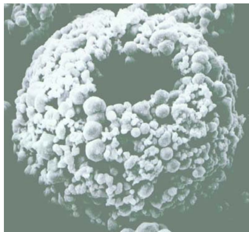
Fig. 1: Morphology of agglomerated and sintered particle of Mo powder /2/.
