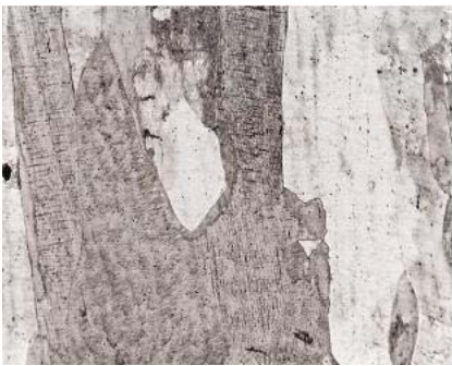
Fig.5: Microstructure of deposited layer for the third pass hardfacing (X 100)
