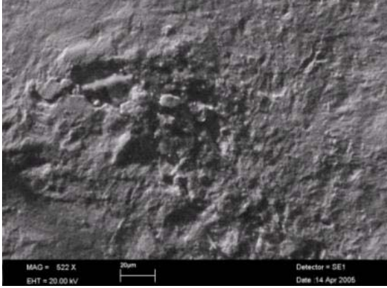
Fig.9: Surface topography of eroded first layer (Impact angle: 90°)
