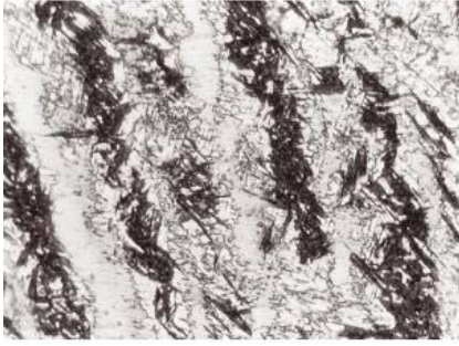
Fig.4: Microstructure of deposited layer for the second pass hardfacing (X 375)
