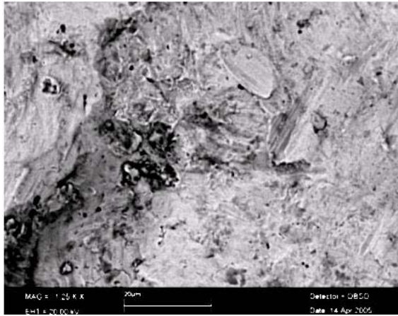
Fig.10: Top view of eroded surface the belonging of third layer deposited. (Impact angle: 30°)
