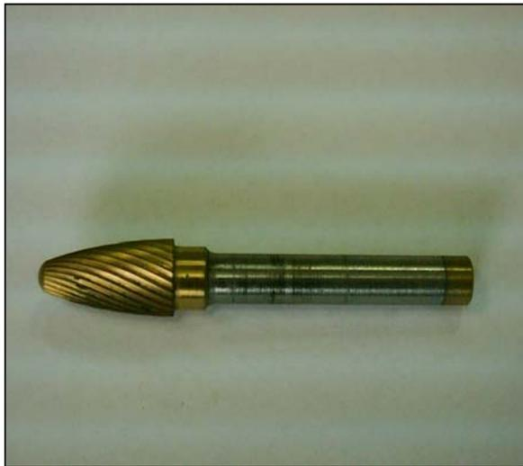
**Fig. 1:** Representation of tooth milling cutter
