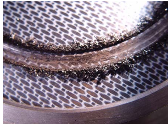
Fig. 10: Wear track of disc PPSA2, after 9000 rounds.
