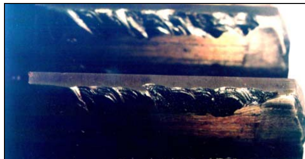
Figure 5: Working surfaces of the teeth hardfaced with additional material UTP 670 after 98 \cdot 10^6 cycles
