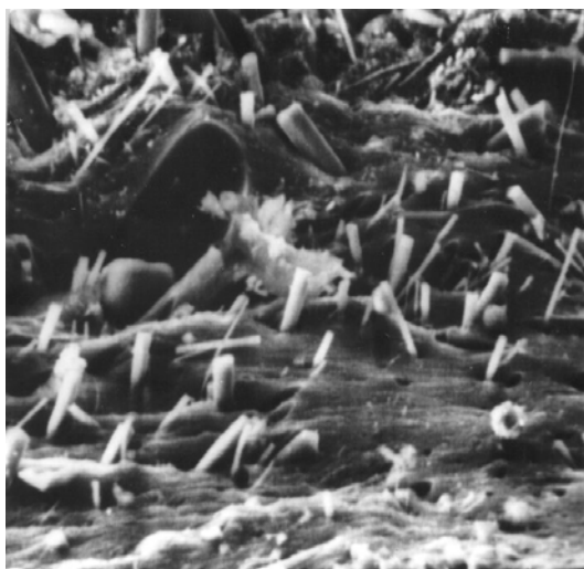
Figure: SEM image of a microporous (a) and orthogonally reinforced (b) structure of FM
