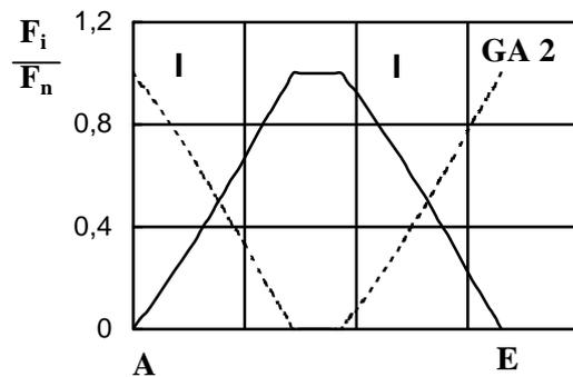
**Figure 2:** Variation of load sharing ratio in meshing cycle
