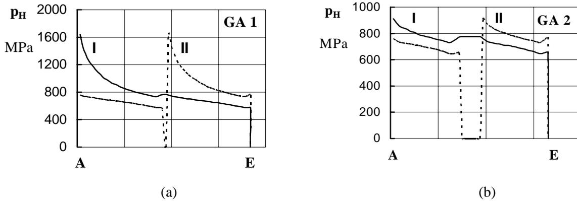
**Figure 3:** Variation of Hertz contact pressure along the equivalent line of action
