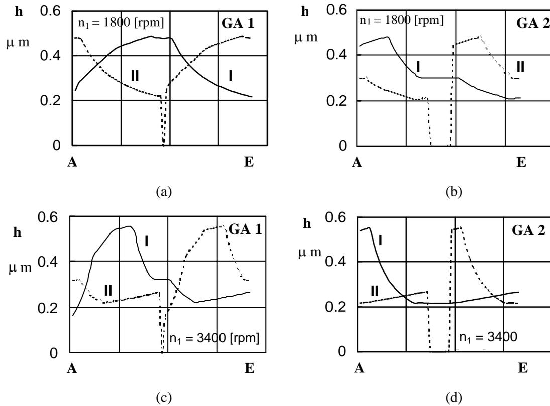
**Figure 5:** Variation of film thickness along the equivalent line of action
