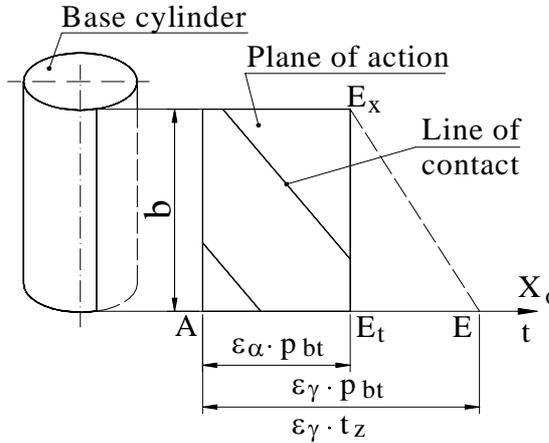
**Figure 1:** Plane of action and the equivalent line of action
