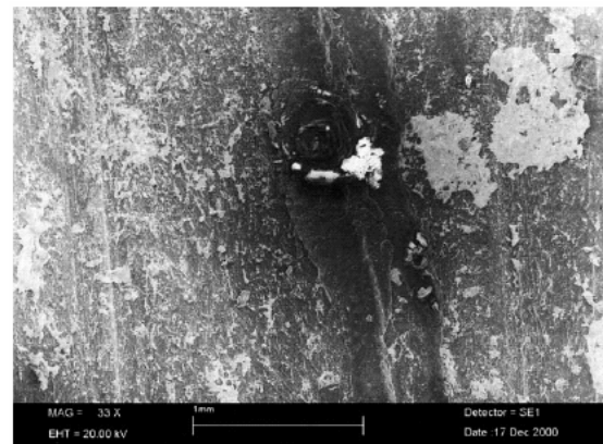
Fig. 3: The SiC particle transferred by rubbing the surface together with projectile [9].
