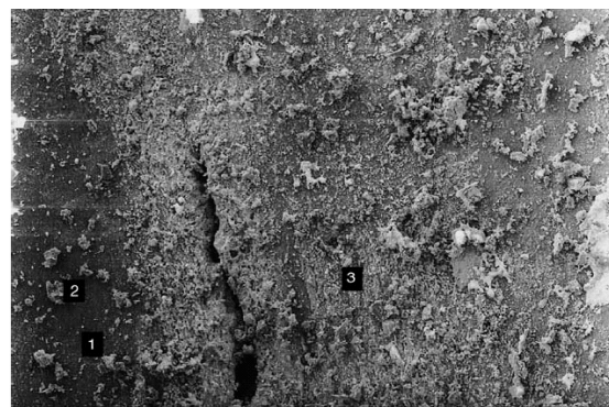
Fig. 5: The fracture surface of the hole (SiCp) [9].
