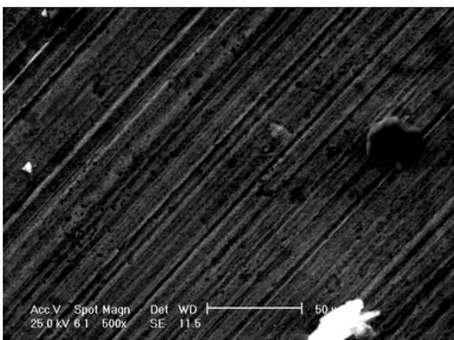
Fig. 19. SEM image showing worn surface of ZA-27 HT5
