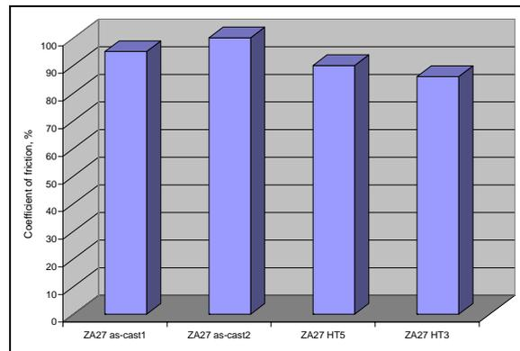
Fig. 15. Coefficients of frictions of alloys underload of  $F_N=100\text{ N}$
