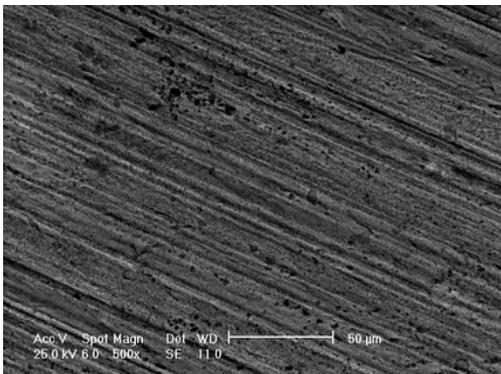
Fig. 18. SEM image showing worn surface of ZA-27 HT3
