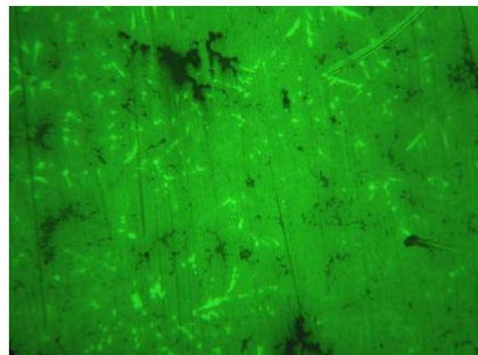
Fig. 7. Microstructure of ZA-27 HT3 (X50)
