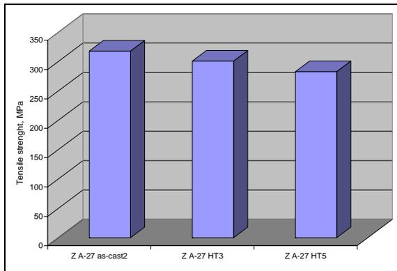
Fig. 3. Heat treatment effects on tensile strength of ZA-27 alloy
