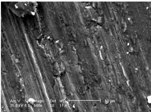
Fig. 17. SEM image showing worn surface of ZA-27 as-cast2 alloy
