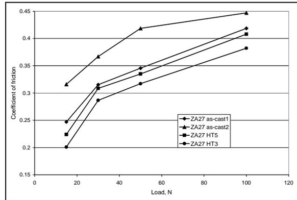
Fig. 12. Average coefficients of friction of alloys for whole sliding time under different loads
