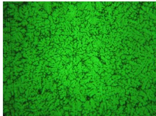
Fig. 6. Microstructure of ZA-27 as-cast2 (X50)
