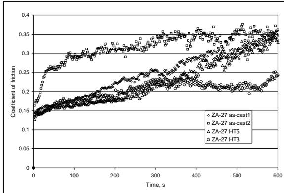
Fig. 10. Coefficients of frictions tested alloys ( $F_N=15\text{ N}$ ,  $v=0,26\text{ m/s}$ )
