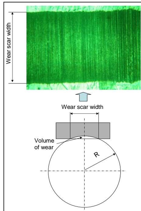
Fig. 2. The contact pair geometry
