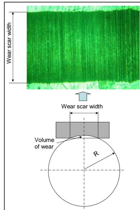
Fig. 2. The contact pair geometry
