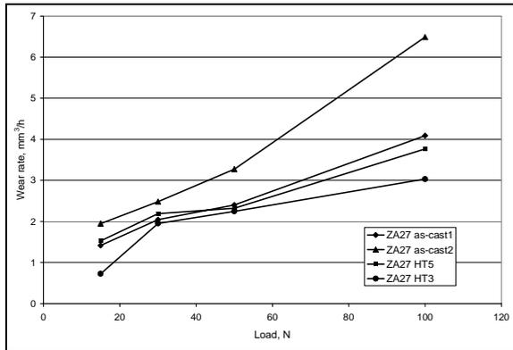
Fig. 13. Wear rates of alloys under different loads
