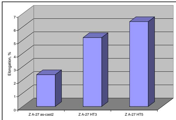
Fig. 4. Heat treatment effects on elongation of ZA-27 alloy
