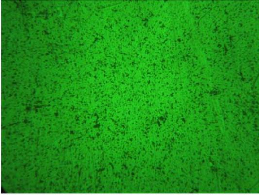
Fig. 8. Microstructure of ZA-27 HT5 (X50)
