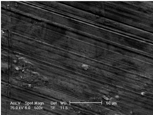
Fig. 16. SEM image showing worn surface of ZA-27 as-cast1 alloy
