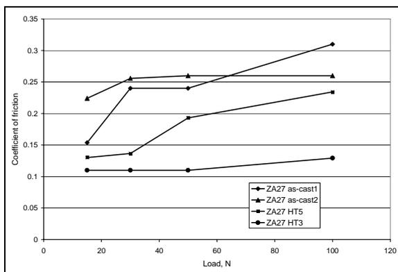
Fig. 11. Average coefficients of friction of alloys for first 60s of sliding under different loads
