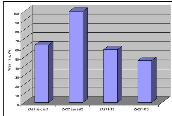
Fig. 14. Wear rates of alloys under load of  $F_N=100\text{ N}$
