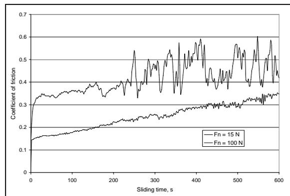
Fig. 9. Examples of friction coefficient variation during sliding time
