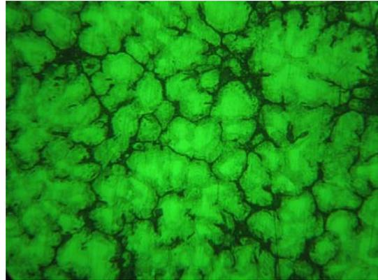
Fig. 5. Microstructure of ZA-27 as-cast1 (X50)
