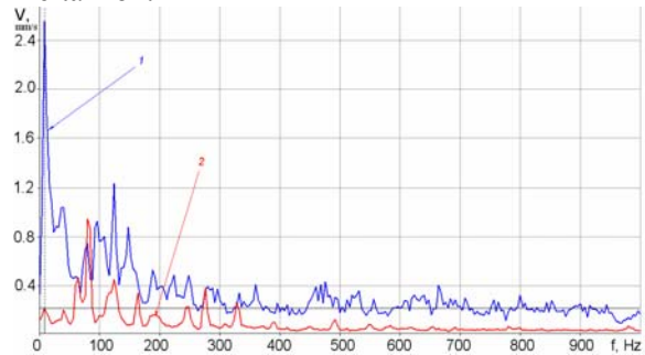
Figure 2 Vibration velocity spectra recorded by laser vibrometer (1) and accelerometer (2)
