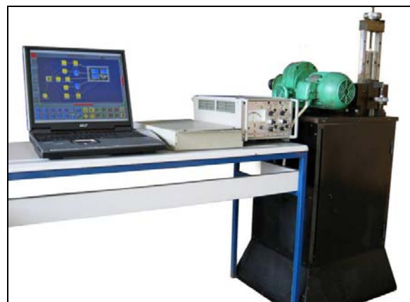
Figure 2. The tribometer with the measurements setup and contact geometry
