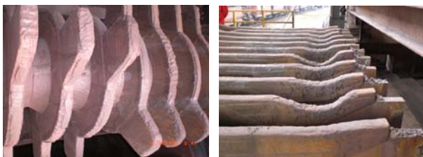
Figure 1. Heavy duty equipment exposed to high temperature abrasion and impact: Sinter crusher rotor and crusher bars
