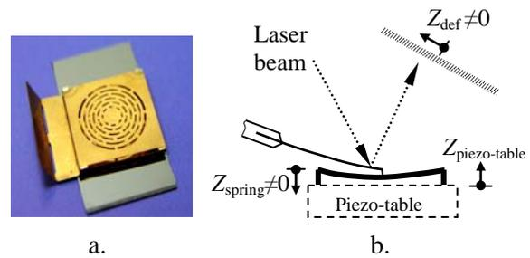
**Figure 4.** Measurement of the stiffness of the cantilever with spherical tip by use a microspring: a. microspring, b. schematic of stiffness measurement
