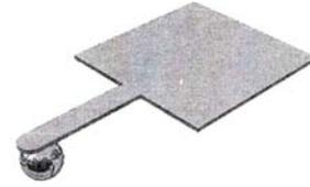
**Figure 3.** AFM cantilever with a sphere as tip
