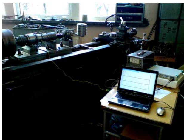
Figure 8. Device for testing three cone bits axial sliding bearings
