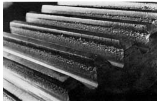
Figure 1. Pitting of gear teeth [11]
