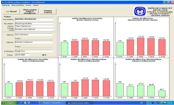
Figure 5. Histogram of machinability index for the group of tough materials
