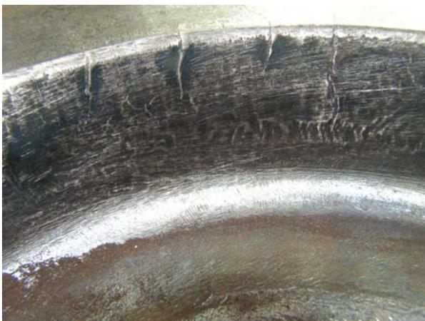
Figure 1. The cracks in the body of die.
