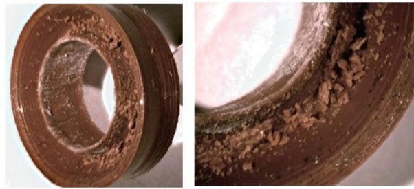
Figure 6. Abrasive wear of the lip due to hard debris
