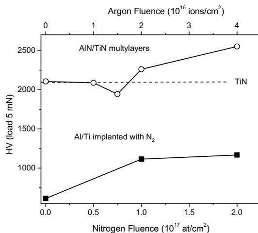
**Figure 6.** Nano-hardness as a function of the irradiation fluence for both (AlN/TiN)<sub>x5</sub>/Si and (Al/Ti)<sub>x5</sub>/Si structures.
