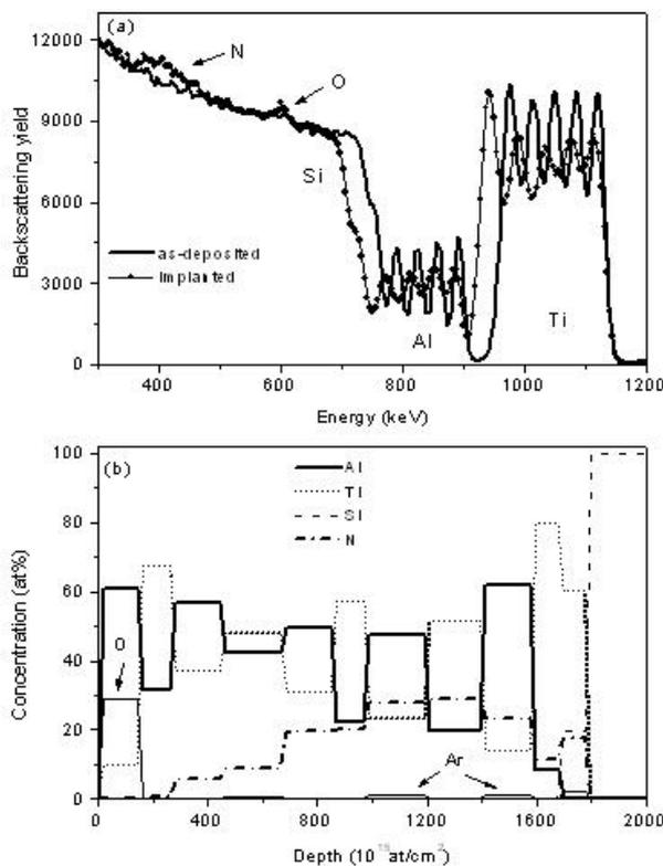
**Figure 2.** RBS analysis of  $(Al/Ti)_x5/Si$ : (a) experimental spectra from an as-deposited sample and sample implanted with nitrogen to  $2 \times 10^{17}$  at/cm<sup>2</sup>; (b) extracted depth profiles of the implanted sample.
