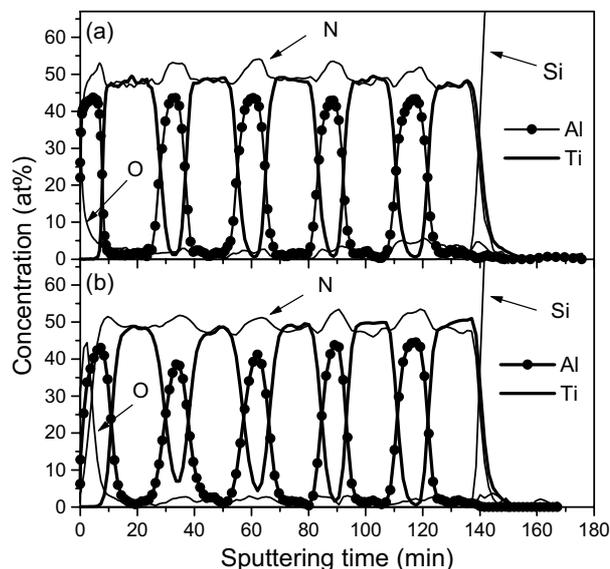
**Figure 1.** XPS depth profiles of (AlN/TiN)<sub>x5</sub>/Si: (a) as-deposited sample; (b) sample implanted with argon to  $4 \times 10^{16}$  ions/cm<sup>2</sup>.
