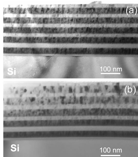
**Figure 4.** Bright field cross-sectional TEM images of: (a) as-deposited  $(AlN/TiN)_x5/Si$ ; (b)  $(AlN/TiN)_x5/Si$  implanted with argon to  $2 \times 10^{16}$  ions/cm<sup>2</sup>.
