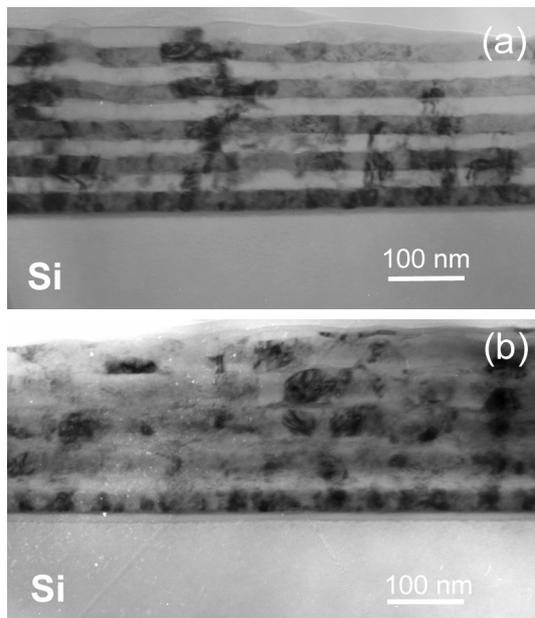
**Figure 5.** Bright field cross-sectional TEM images of: (a) as-deposited (Al/Ti)<sub>x5</sub>/Si; (b) (Al/Ti)<sub>x5</sub>/ implanted with nitrogen to  $2 \times 10^{17}$  at/cm<sup>2</sup>.
