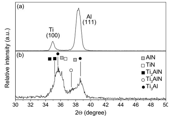
**Figure 3.** XRD spectra: (a) from as-deposited  $(Al/Ti)_x5/Si$ ; (b) sample implanted with nitrogen to  $2 \times 10^{17}$  at/cm<sup>2</sup>.
