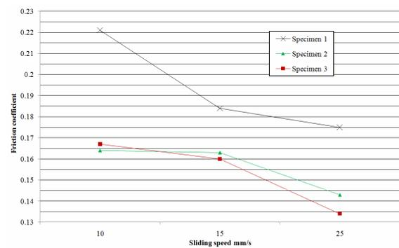
**Figure 2.** Friction coefficient of TiN coatings with different roughness in function of sliding speed
