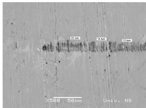
**Figure 3.** SEM micrograph of worn channel generated on Specimen 2,  $F=100\text{mN}$ ,  $v=10\text{mm/s}$
