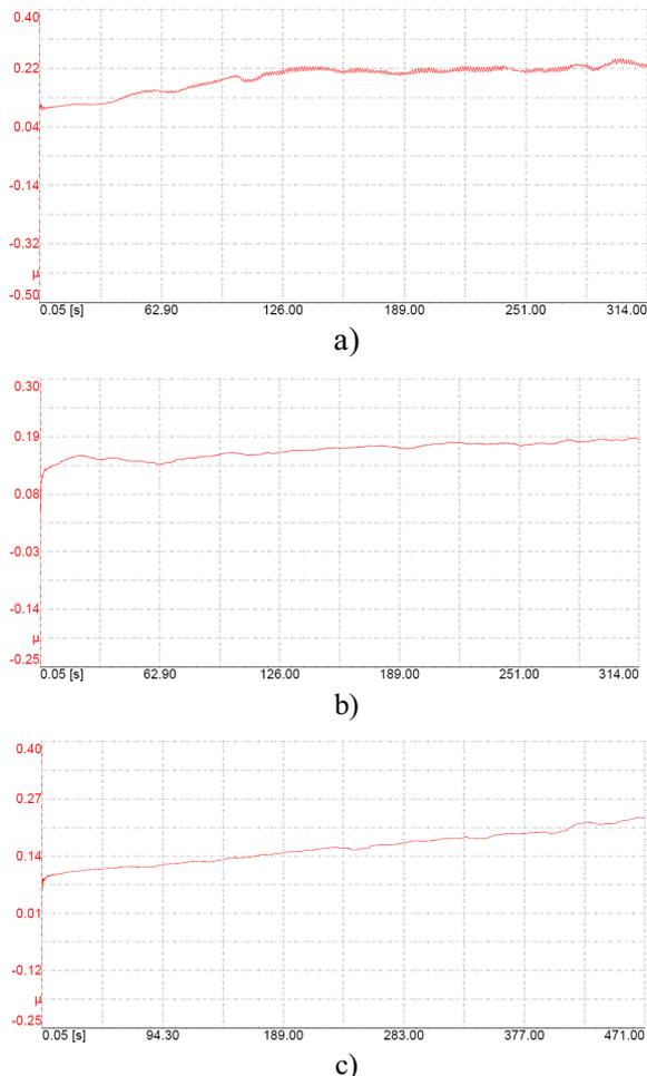
**Figure 1.** Evolution of the friction coefficient for different specimens,  $v=15\text{mm/s}$ ,  $F=100\text{mN}$
