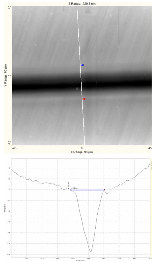
**Figure 5.** Measurement of wear track width
