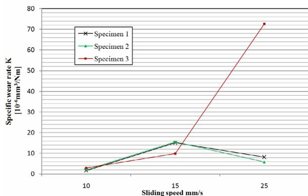
**Figure 6.** Specific wear rate of TiN coatings with different roughness in function of sliding speed
