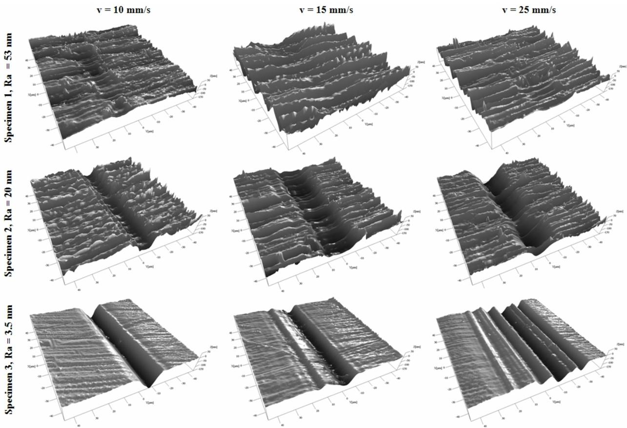
**Figure 4.** Morphology of the worn zones generated on TiN coatings of different roughness by reciprocating sliding with different sliding speeds
