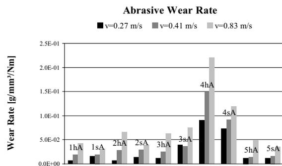
Figure 11. Abrasive wear rate, A materials - perpendicular
