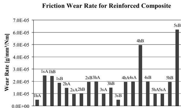
Figure 10. Friction wear rate – parallel sliding
