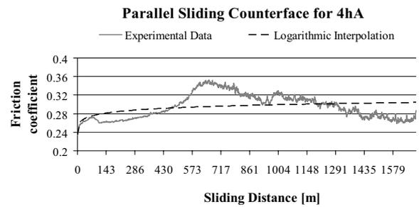
**Figure 5.** Friction coefficient of 4hA material
