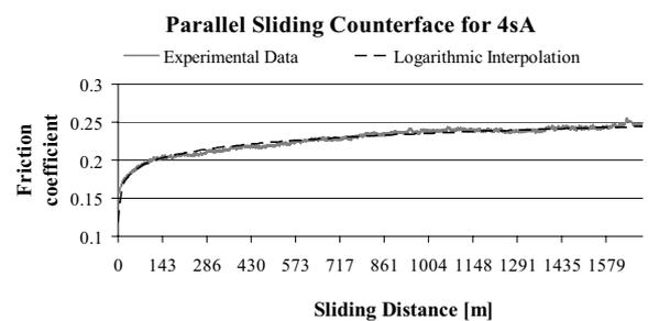
**Figure 7.** Friction coefficient of 4sA material
