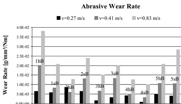
Figure 14. Abrasive wear rate, B materials - parallel
