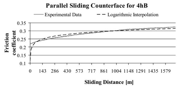
**Figure 6.** Friction coefficient of 4hB material
