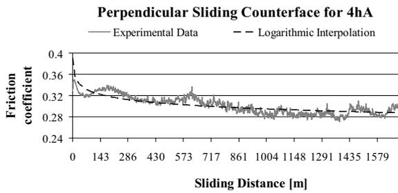
**Figure 1.** Friction coefficient of 4hA material
