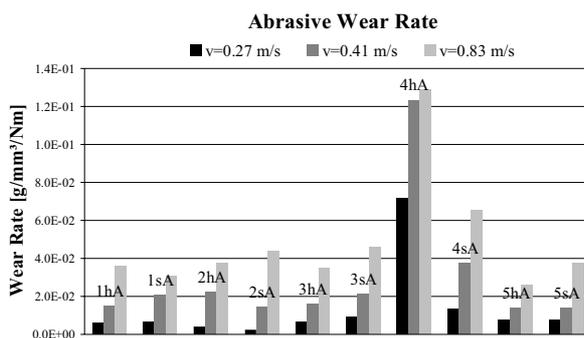
Figure 13. Abrasive wear rate, A materials - parallel
