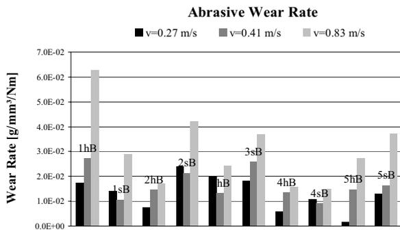
Figure 12. Abrasive wear rate, B materials - perpendicular
