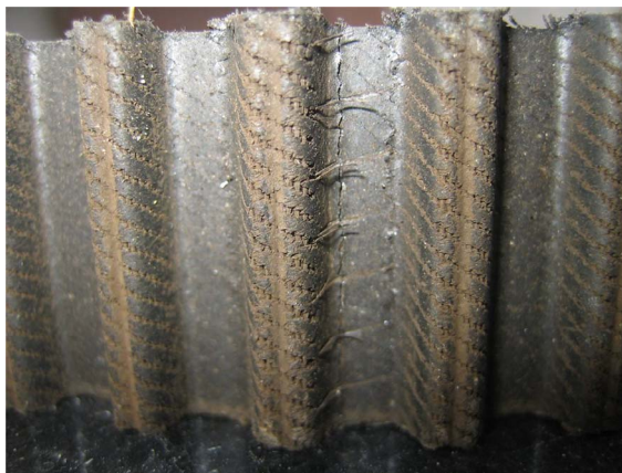
Figure 5. Damage of the face surface of the belt
