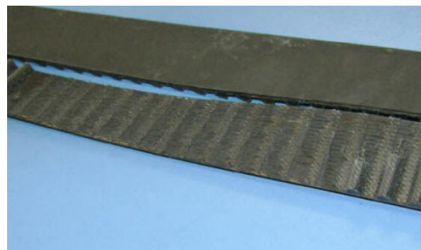
Figure 4. Cutting off of larger number of the belt's teeth
