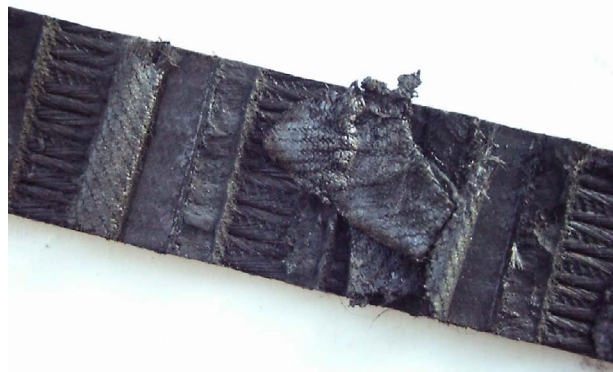
Figure 6. Influence of the oil and solvents on belt
