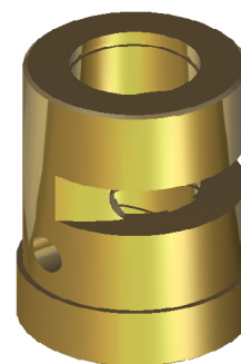
Figure 10. 3D CAD model of Tesla's radial slide bearing T: 23.102
