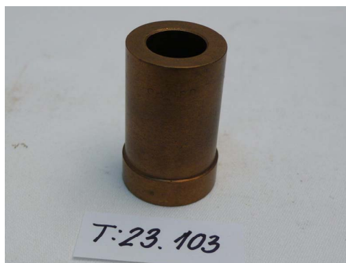
Figure 4. Machined piece for slide bearing T:23.103 (Collection of Objects from the Field of Mechanical Engineering)
