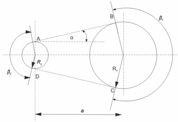
**Figure 3.** Schematic of ideal metal belt geometry
