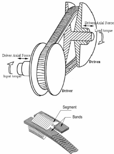
**Figure 2.** Schematic diagram of a metal-pushing CVT, or a metal V-belt drive
