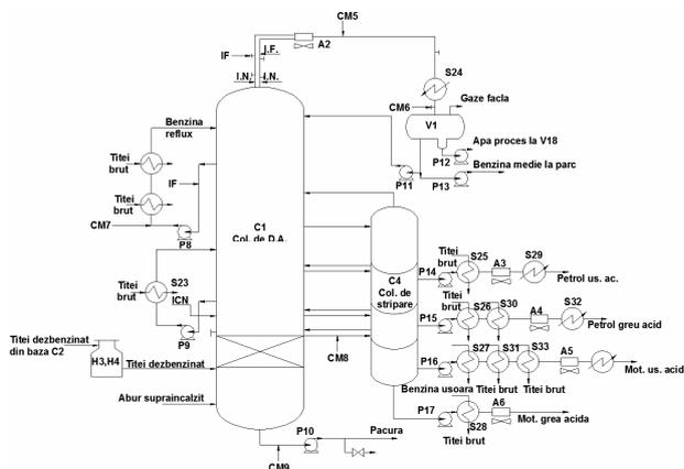
**Figure 1** The technological scheme of the atmospheric distillation of crude oil plant
