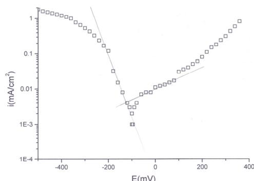
**Figure 5** Polarization curves of steel in the austenitic X6CrNiMoTi 17-12-2 condensate from the top 1% DV column naphthenic acids.
