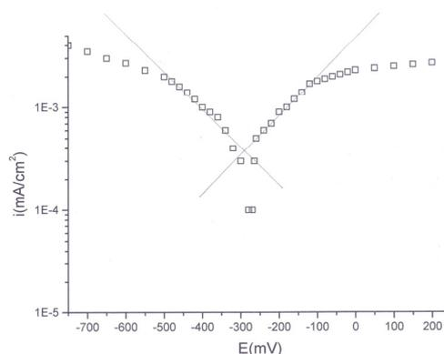
**Figure 6** Polarization curves of austenitic steel X6CrNiMoTi 17-12-2 in condensation on top of the column with 1% DV naphthenic acids.
