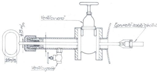
**Figure 3.** Device with retractable probe for corrosion measurement
