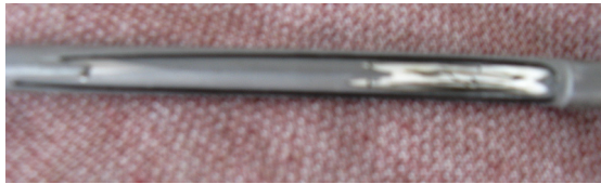
Figure 2. Eroded PT 100 sensor
