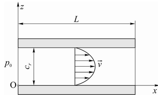
**Figure 4.** The flow of fluid between parallel plates
