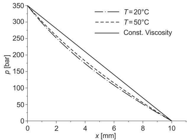
**Figure 5.** Change of pressure along the clearance
