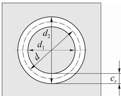
**Figure 3.** Symmetric radial clearance
