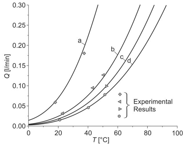
**Figure 7.** Theoretical curves: a) overlap 2 mm, b) overlap 6 mm; a) overlap 8 mm; a) overlap 10 mm
