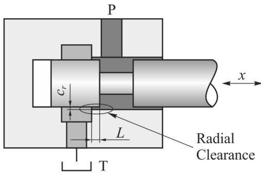
**Figure 2.** Flow of hydraulic fluid through long radial clearance
