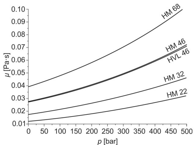
**Figure 2.** Change of viscosity of some mineral hydraulic oils with the change of pressure (temperature 50 °C) [4]
