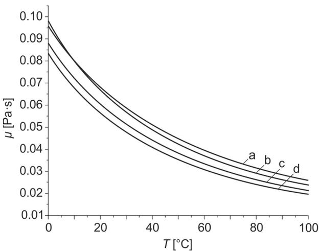
**Figure 6.** Temperature-viscosity coefficient of hydraulic oil: a) HM 68; b) HM 46; c) HM 32; d) HM 22
