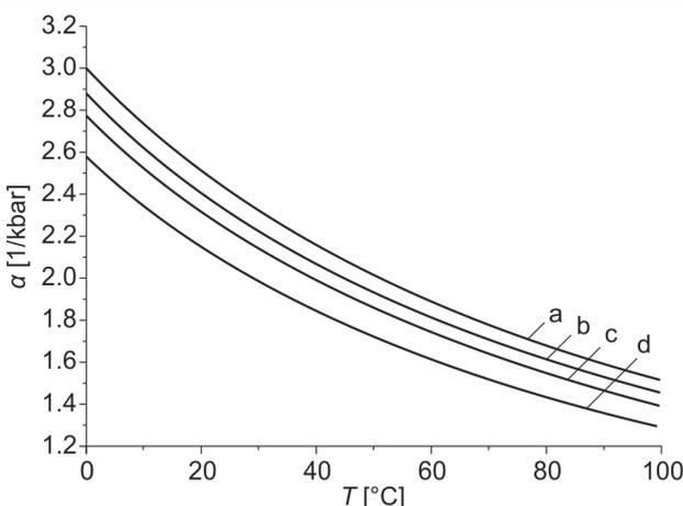
**Figure 1.** Pressure-viscosity coefficient of mineral oil paraffinic base structure: a)  $p = p_a$ ; b)  $p = 500$  bar; c)  $p = 1000$  bar; d)  $p = 2000$  bar
