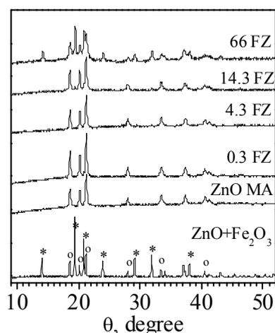
**Figure 1.** XRD patterns of the  $\text{Fe}_2\text{O}_3$ -ZnO sample. The mark (\*) indicated the peaks corresponding to  $\text{Fe}_2\text{O}_3$ , and the marks (o) – peaks corresponding to ZnO.
