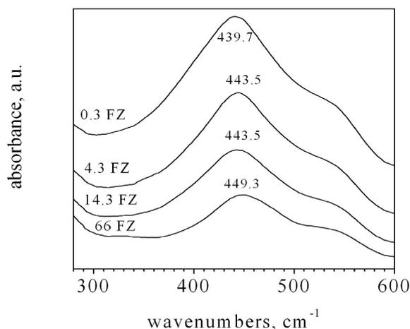
**Figure 2.** FTIR spectra of the  $\text{Fe}_2\text{O}_3$ -ZnO mixed oxides
