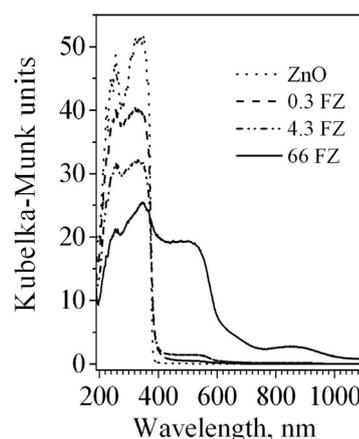
**Figure 3.** UV-vis diffuse reflectance spectra of ZnO and  $\text{Fe}_2\text{O}_3$ -ZnO mixed oxides
