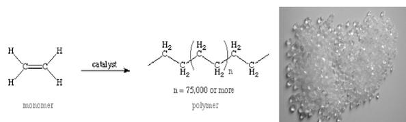
**Figure 2.** Left: The repeating unit of polyethylene; Right: Granulated polyethylene.
