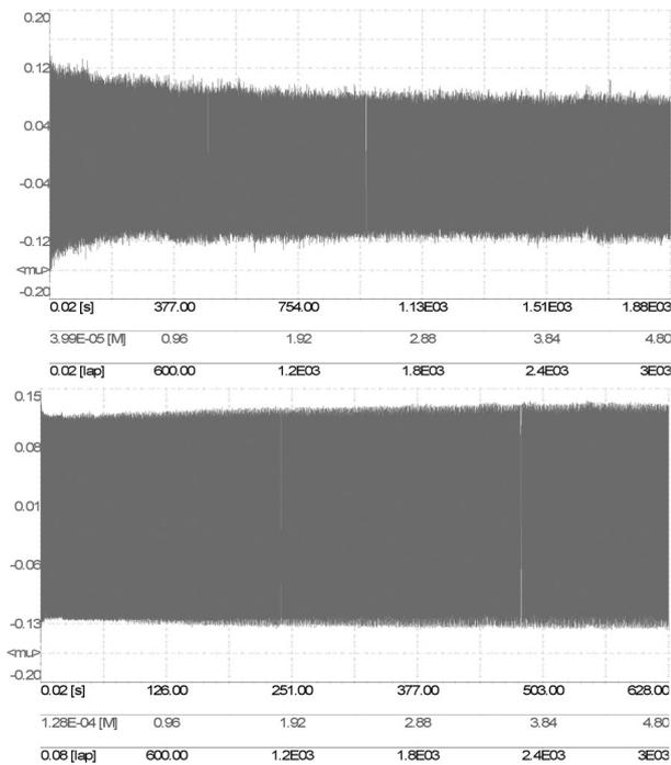
**Figure 3.** Dynamic friction coefficient curve during dry sliding: a)  $v=4$  mm/s,  $F_N=100$ mN; b)  $v=12$  mm/s,  $F_N=1000$ mN.
