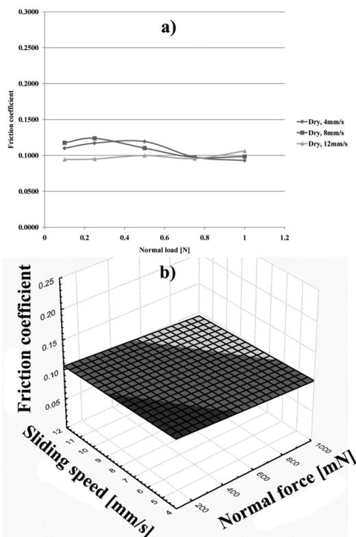
**Figure 4.** a) Friction coefficient as a function of the normal load; b) Friction coefficient as a function of the normal load and sliding speed.
