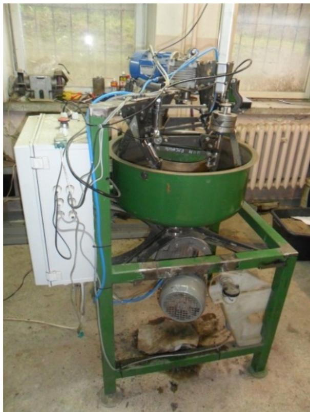
**Figure 1.** Photo of wear machine "spinning mass" type
