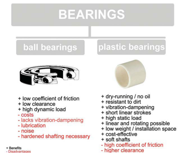
Figure 3. Comparing ball bearings to plastic bearings
