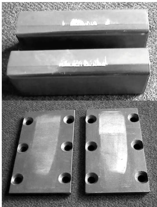
Figure 4. Aluminum glued particles on die and puncher surfaces
