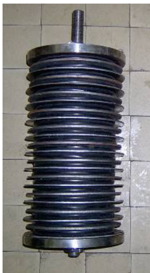
Figure 1. Rubber-metal spring assembly of buffing gear
