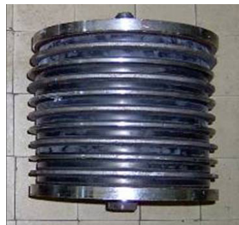
Figure 2. Rubber-metal spring assembly of draw gear
