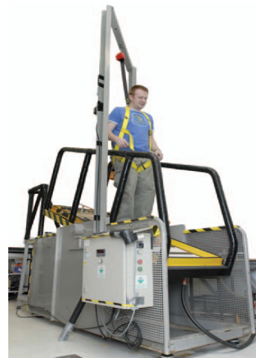
Figure 3. The ramp friction coefficient test
