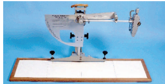
Figure 2. The pendulum friction coefficient test
