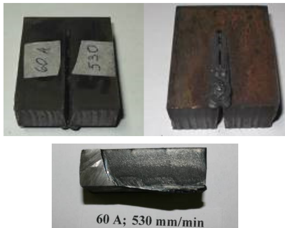
Figure 12. Cutting with 530 mm/min and 60 A
