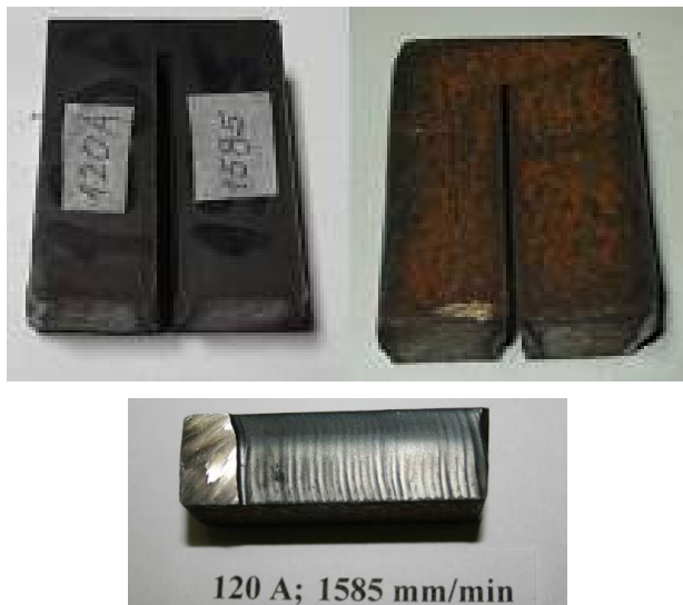
Figure 15. Cutting with 1585 mm/min and 120 A
