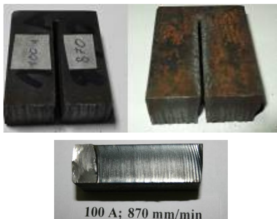
Figure 14. Cutting with 870 mm/min and 100 A
