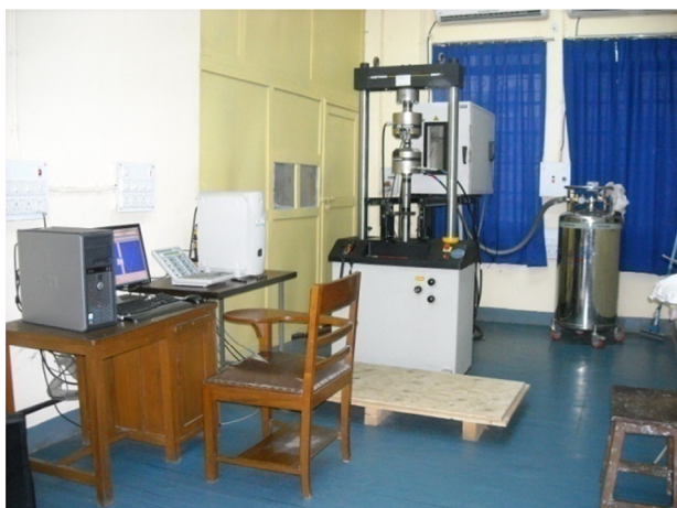
Figure 2. 'Instron' equipped with data acquisition software.
