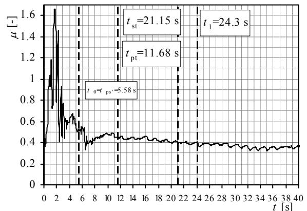
Figure 4. Friction coefficient: “theoretical” welding tool,  $n=265$  rpm,  $d_0=5$  mm
