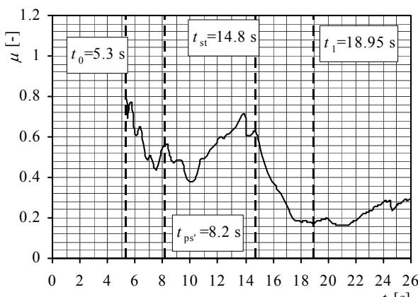
**Figure 20.** Friction coefficient: CWT,  $n=600$  rpm,  $d_0=0$  mm
