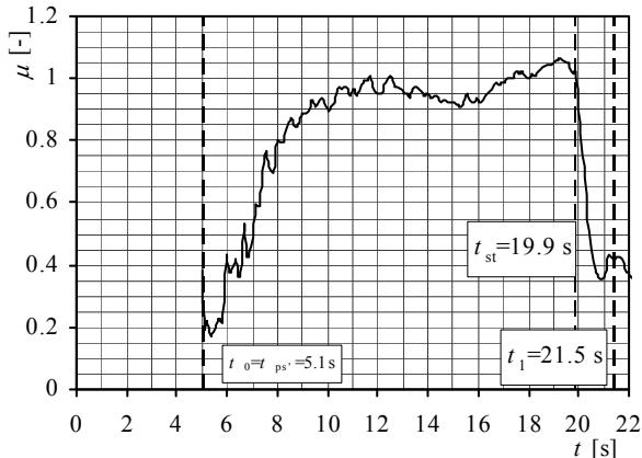
**Figure 14.** Friction coefficient: CWT,  $n=600$  rpm,  $d_0=5$  mm
