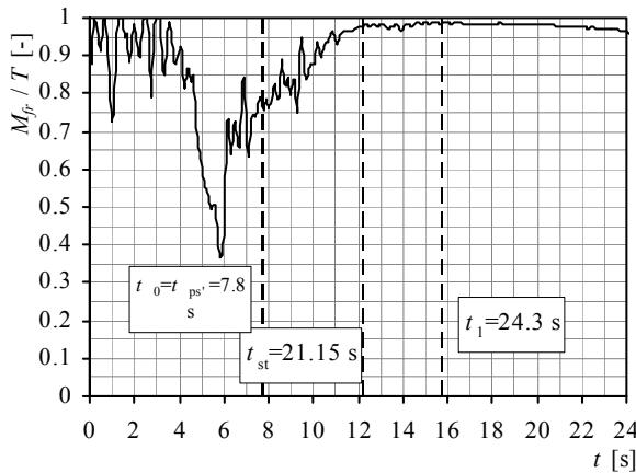
**Figure 23.** Ratio  $M_f/T$ : CWT,  $n=910$  rpm,  $d_0=5$  mm
