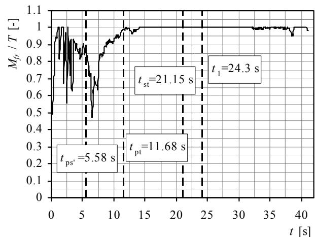
Figure 5. Ratio of the momentum of friction and the torque: “theoretical” welding tool,  $n=265$  rpm,  $d_0=5$  mm
