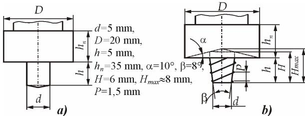
Figure 2. Welding tool
