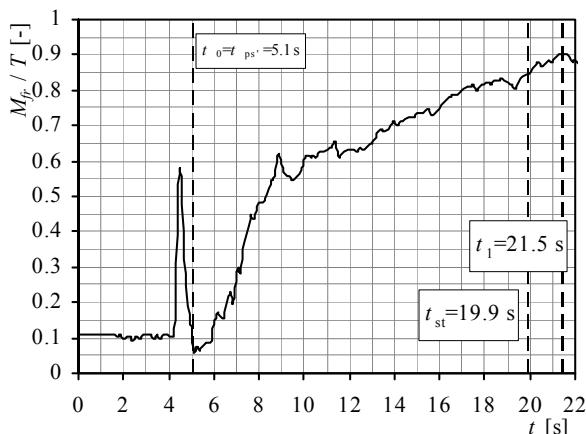
**Figure 15.** Ratio  $M_{fr}/T$ : CWT,  $n=600$  rpm,  $d_0=5$  mm
