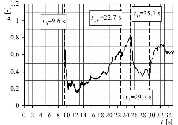
**Figure 10.** Friction coefficient: CWT,  $n=265$  rpm,  $d_0=2$  mm
