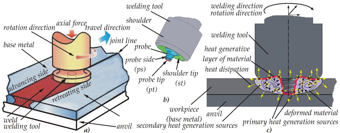
**Figure 1.** Friction stir welding
