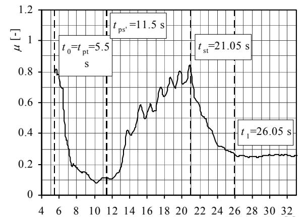
**Figure 28.** Friction coefficient: CWT,  $n=910$  rpm,  $d_0=0$  mm
