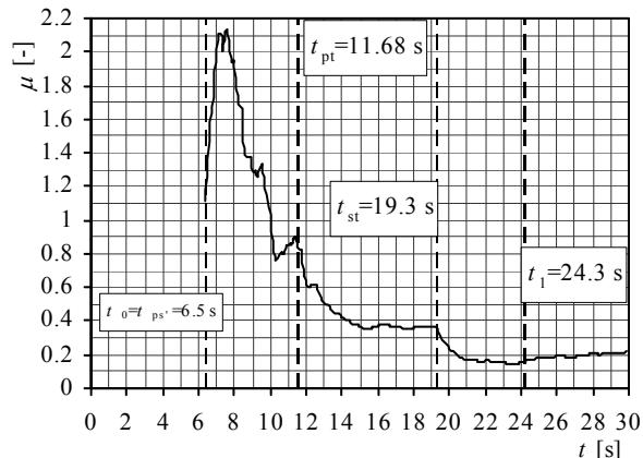
**Figure 18.** Friction coefficient: CWT,  $n=600$  rpm,  $d_0=2$  mm
