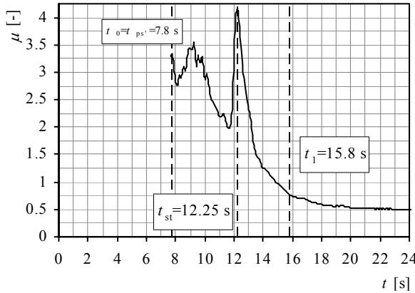
**Figure 22.** Friction coefficient: CWT,  $n=910$  rpm,  $d_0=5$  mm
