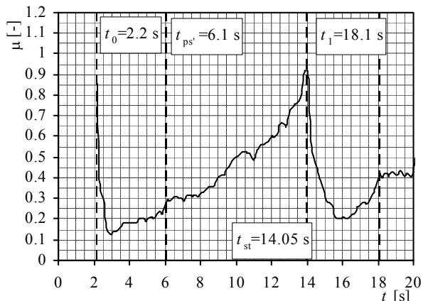
**Figure 12.** Friction coefficient: CWT,  $n=265$  rpm,  $d_0=0$  mm
