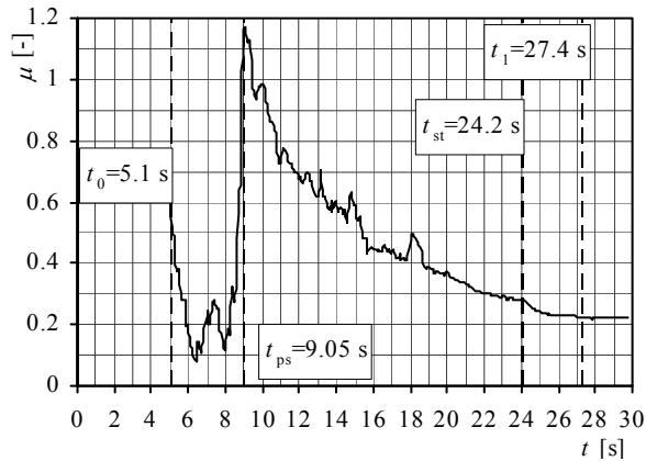
**Figure 6.** Friction coefficient: CWT,  $n=265$  rpm,  $d_0=5$  mm
