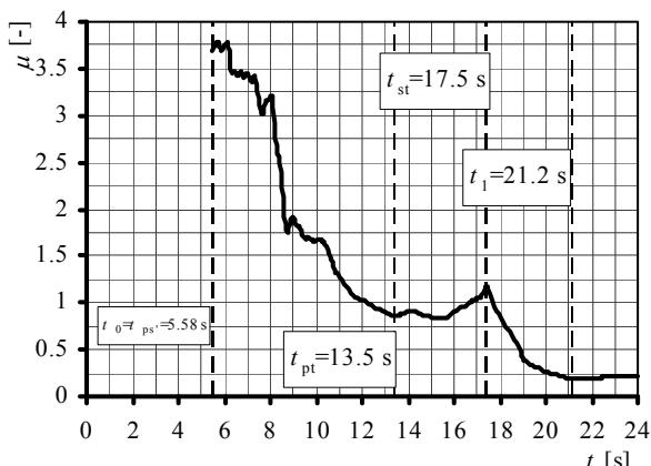
**Figure 16.** Friction coefficient: CWT,  $n=600$  rpm,  $d_0=3.2$  mm
