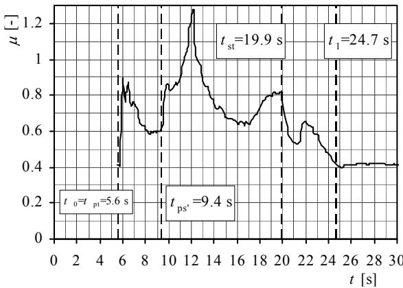
**Figure 24.** Friction coefficient: CWT,  $n=910$  rpm,  $d_0=3.2$  mm
