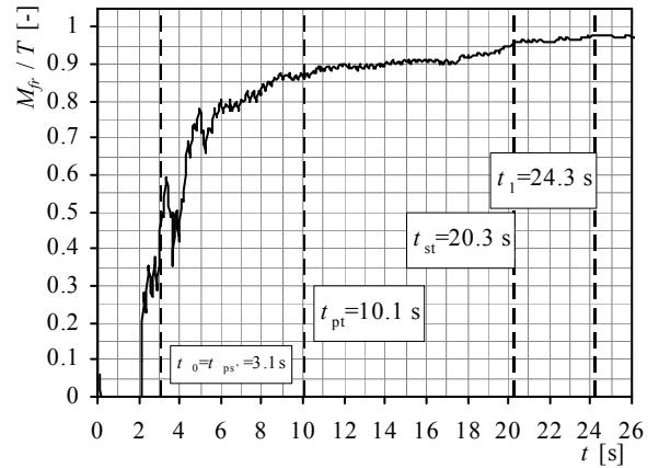
**Figure 9.** Ratio of the momentum of friction and the torque: CWT,  $n=265$  rpm,  $d_0=3.2$  mm
