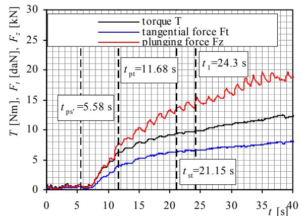
Figure 3. Diagram of measured loads: “theoretical” welding tool,  $n=265$  rpm,  $d_0=5$  mm
