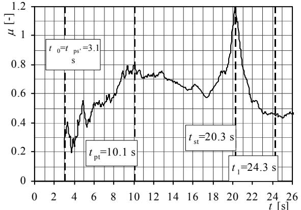
**Figure 8.** Friction coefficient: CWT,  $n=265$  rpm,  $d_0=3.2$  mm
