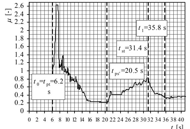
**Figure 26.** Friction coefficient: CWT,  $n=910$  rpm,  $d_0=2$  mm
