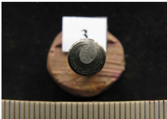
Figure 6. Macrophotography of the wear surface of sample 3 (RT2) after testing
