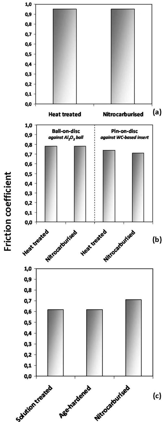
**Figure 3.** Friction coefficient values for various tribosystems: (a) steel (A) against Al<sub>2</sub>O<sub>3</sub> ball, (b) steel (B) against Al<sub>2</sub>O<sub>3</sub> ball and against WC-based insert and (c) steel (E) against WC-based insert
