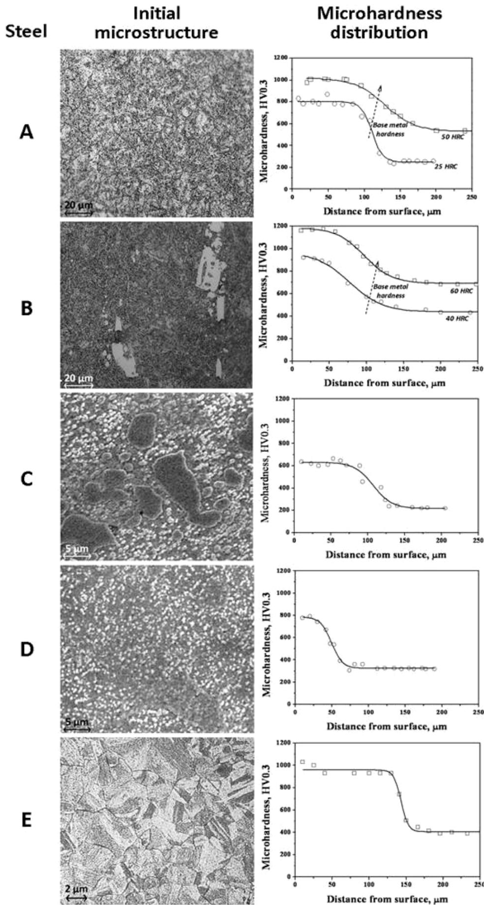
**Figure 2.** Initial microstructure and in-depth microhardness distribution after nitrocarburising of the five (5) steel grades examined
