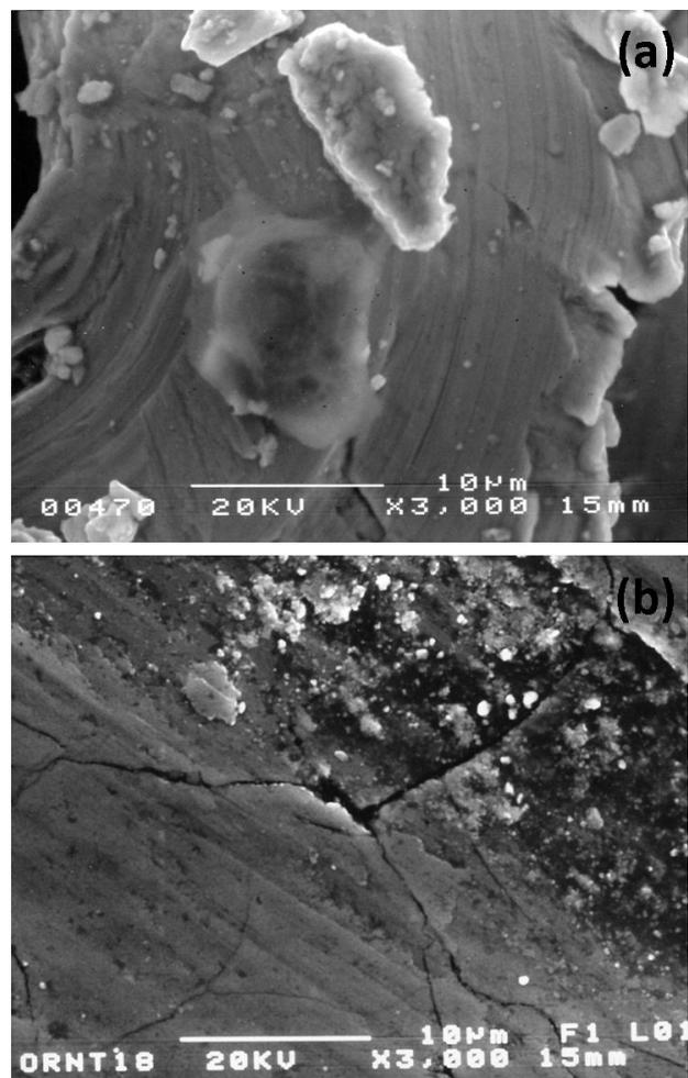
**Figure 9.** Characteristic micrographs of the contact surfaces after steel-on-steel plane contact sliding tests: (a) worn surface of soft-annealed steel (C) showing deformation patterns, (b) worn surface of nitrocarburised steel (C); branched cracks appeared as a precursor of exfoliation and spalling
