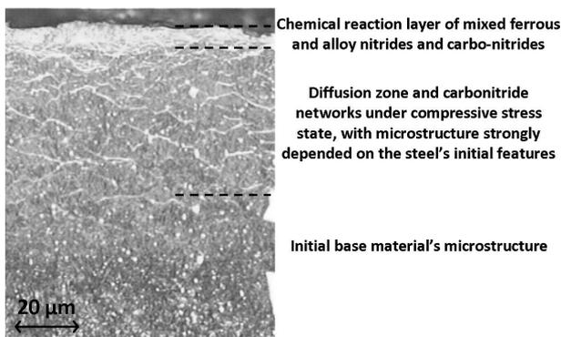
**Figure 1.** Typical microstructure layers of a nitrocarburised tool steel
