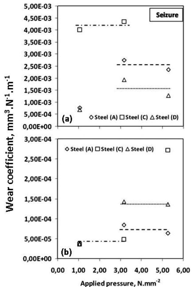
**Figure 7.** Evolution of wear coefficient of the three steel grades examined in conformal configuration (III) versus the applied pressure: (a) in soft-annealing state, (b) after nitrocarburising
