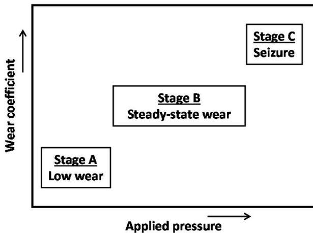
**Figure 8.** Schematic of the wear coefficient evolution versus the applied pressure, for steel-on-steel plane contact sliding
