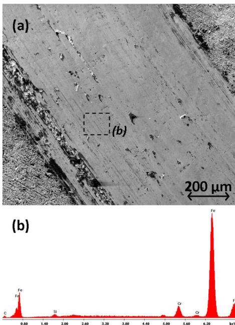
**Figure 6.** (a) Characteristic SEM micrograph of the worn surface of nitrocarburised steel (A), tested in configuration (II) and (b) EDS spectrum of the area marked in (a)
