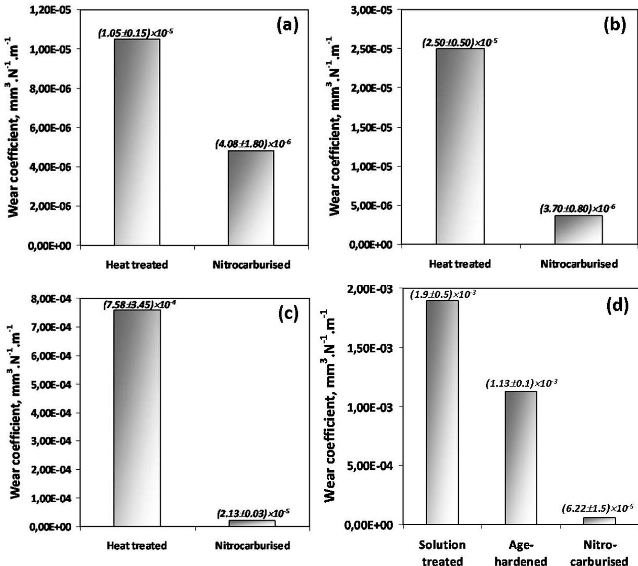
Figure 4. Wear coefficient values for various tribosystems: (a) steel (A) against Al<sub>2</sub>O<sub>3</sub> ball, (b) steel (B) against Al<sub>2</sub>O<sub>3</sub> ball, (C) steel (B) against WC-based insert and (c) steel (E) against WC-based insert
