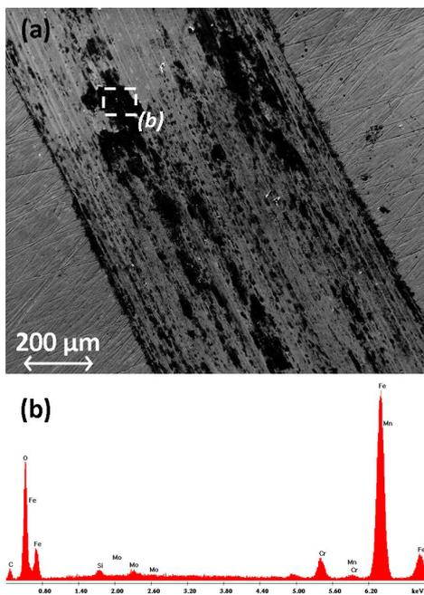
**Figure 5.** (a) Characteristic SEM micrograph of the worn surface of heat-only-treated steel (A), tested in configuration (I) and (b) EDS spectrum of the area marked in (a)
