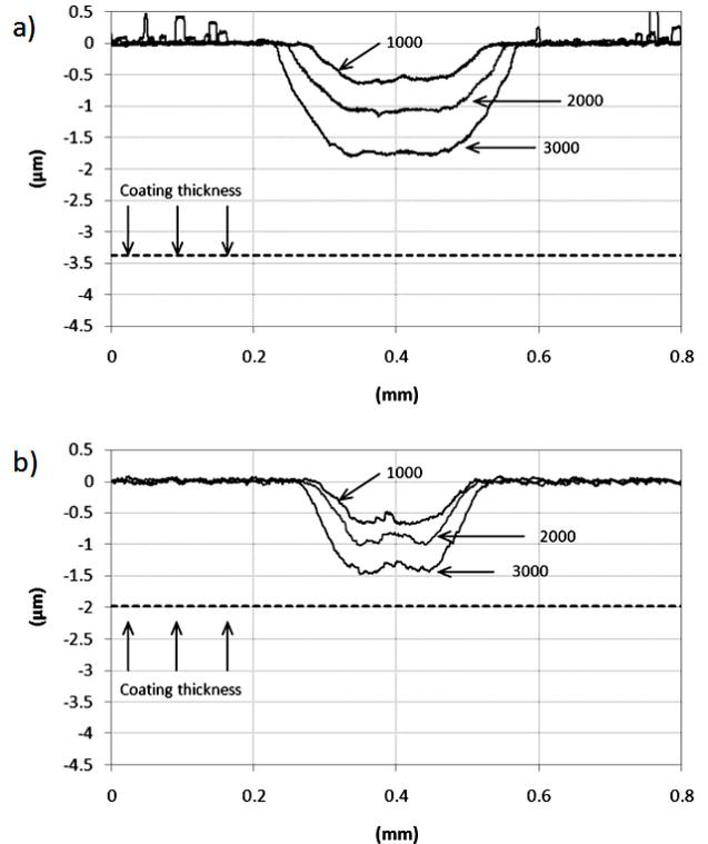
**Figure 3.** 2D wear track profiles of: (a) TiAlN and (b) TiAlN/TiSiN coating
