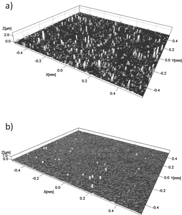
**Figure 1.** 3D surface topography of: (a) TiAlN and (b) TiAlN/TiSiN coating
