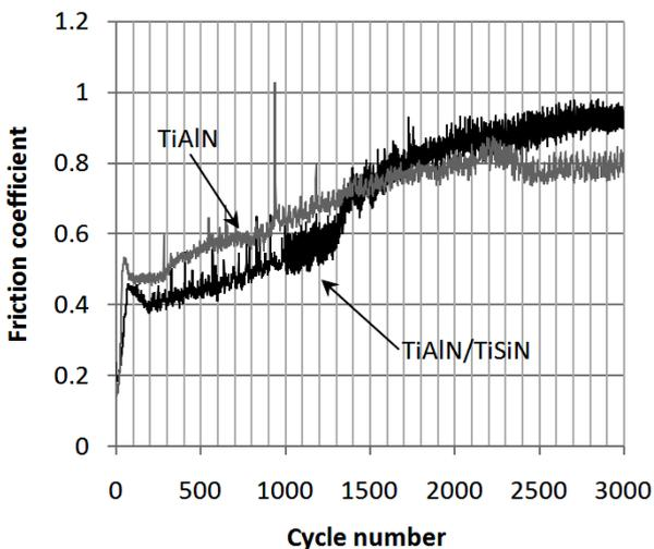
**Figure 2.** Friction curves of TiAlN and TiAlN/TiSiN coating
