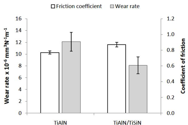
**Figure 4.** Wear rate and friction coefficient of TiAlN and TiAlN/TiSiN coating
