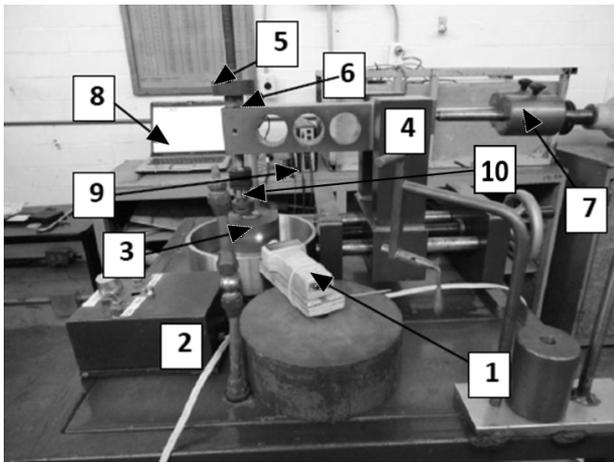
**Figure 2.** Pin-on-disk tester
