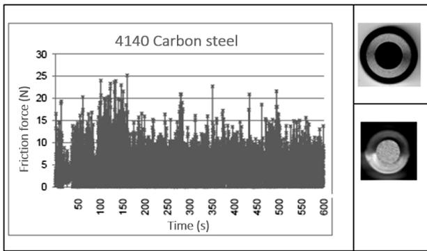
**Figure 4.** Friction force of the 4140 carbon steel pin specimen uncoated as function of the time [18]
