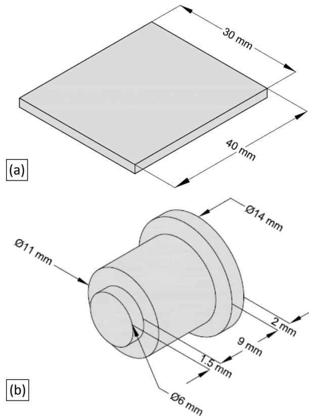
**Figure 1.** Specimens for: (a) corrosion test and (b) sliding wear tests
