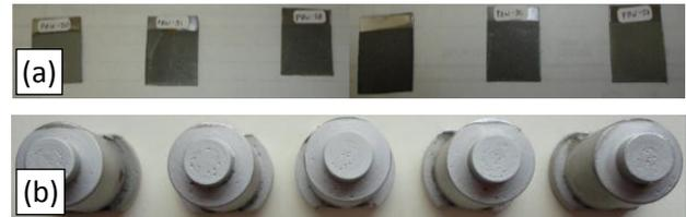
**Figure 3.** Specimens coated for: (a) corrosion test and (b) tribology test
