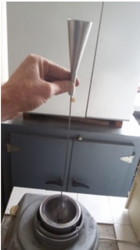
Figure 1. Vibration filling of cored wires
