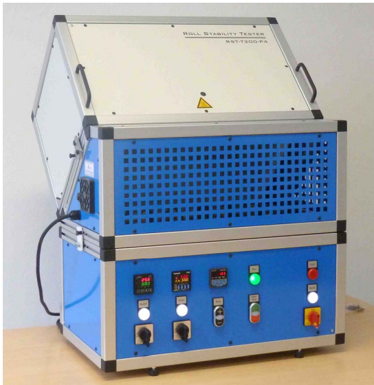
Figure 3. Roll stability tester with room temperature cover
